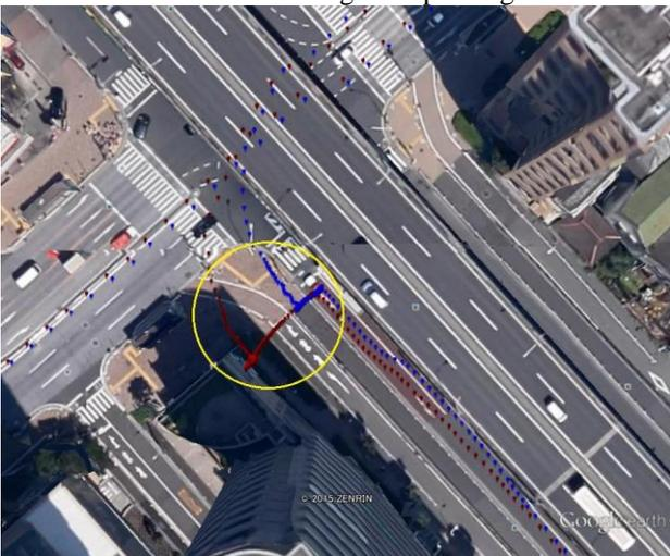
Figure 11 Comparison of horizontal plots between moving antenna and static antenna
