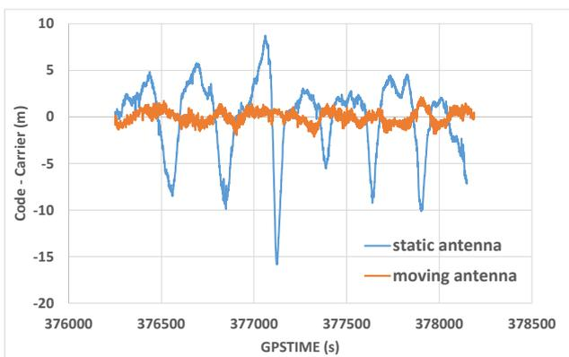
Figure 7 Code-minus-carrier comparison between moving antenna and static antenna (QZS)
