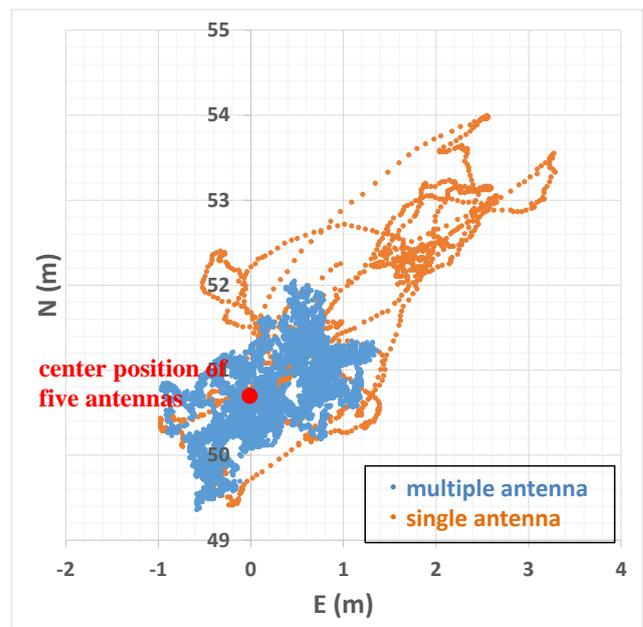
Figure 15 Comparison of horizontal position between the single antenna and the switched multiple antenna
