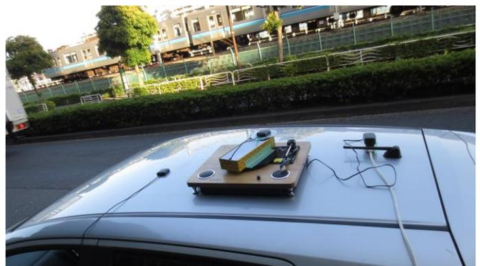
Figure 5 Configuration of two antennas
