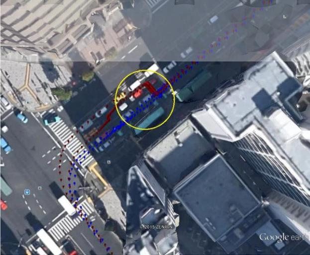
Figure 10 Comparison of horizontal plots between moving antenna and static antenna
