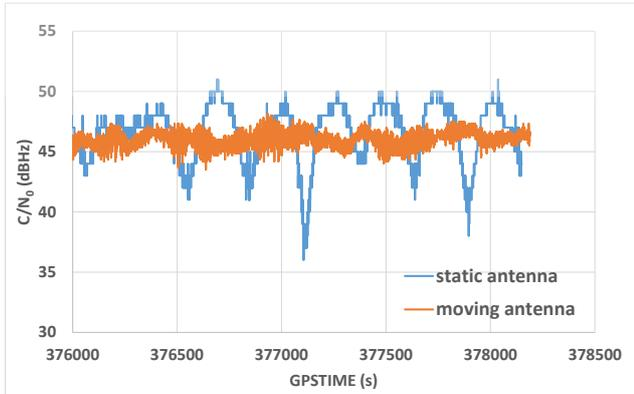
Figure 6 C/N0 comparison between moving antenna and static antenna (QZS)
